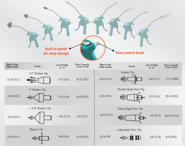
• Working presure: 6.2 Bar ( 90 PSI) • Max. Pressure: 9.8 Bar (142 PSI) • Flow Capacity @ 90 PSI • Air inlet: 1/4"
