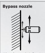
When fore-end air flow is blocked, pressure released through side outlet; reducing pressure for user safety.
