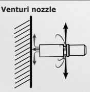
Air flow increases when passes through nozzle. Ambient air is drawn in side ports increases air velocity and volume for extra-high flow. Pressure released through side outlet for user protection when fore-end air flow blocked.
